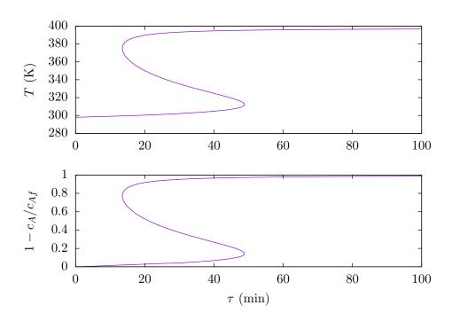
Figure 3: Steady-state solution versus reactor residence time. Note that there are three steady states for residence time in the interval  $15 \le \tau \le 50$ .
