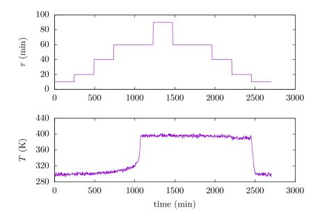
Figure 1: Run of Reactor 1 with changing residence time. Top: reactor residence time versus time. Bottom: reactor temperature versus time.
