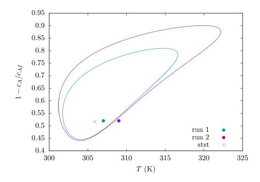
Figure 4: The  $x_A$ , T phase plane. The outer limit cycle is stable; the inner limit cycle is unstable; the steady state is also stable. Initial conditions inside the unstable limit cycle (run 1) are attracted to the stable steady state. Initial conditions outside the unstable limit cycle (run 2) are attracted to the stable limit cycle.
