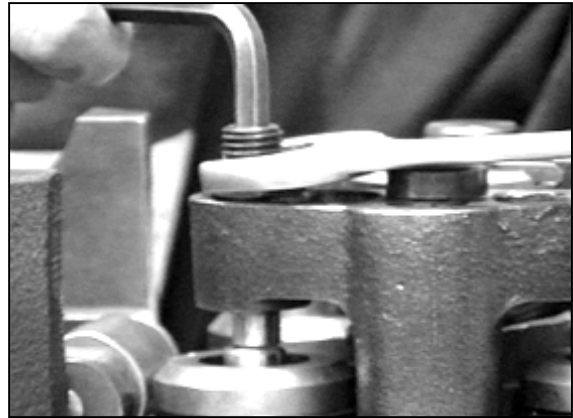
Fig.5 Set the adjuster on the bridge pieces so both will open simultaneously.
