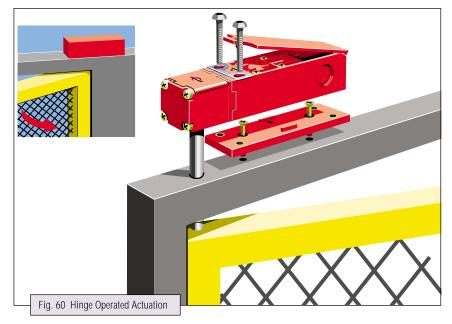
mechanism to the control circuit contacts (*fig. 60*). *Features:*
