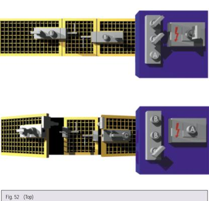
Double access guard doors interlocked with the Power Isolation Switch. Key "A" is trapped in the isolation switch. Both "B" keys are trapped in a Key Exchange Unit. Power is ON and there is no access available to the machine through the locked guard doors.
