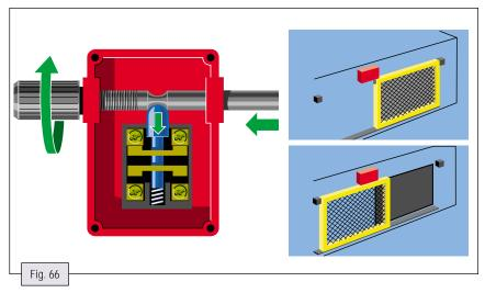
able and it must not be possible for the bolt to be withdrawn before the hazard has ceased. It must only be possible to extend the bolt into its locked position when the guard is fully closed. This means that it will usually be necessary to install stops to restrict the travel of the guard door.
