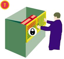
Fig. 56 Use an interlocking device with guard locking to prevent guard opening before the hazard has ceased.
