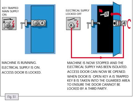
position. When the key is turned the isolation switch contacts are locked open (isolating the power supply) and the key can be withdrawn. The guard door is locked closed and the only way to unlock it is by using the key from the isolator. When this key is turned to release the guard locking unit it is trapped in position and cannot be removed until the guard is closed and locked again.
