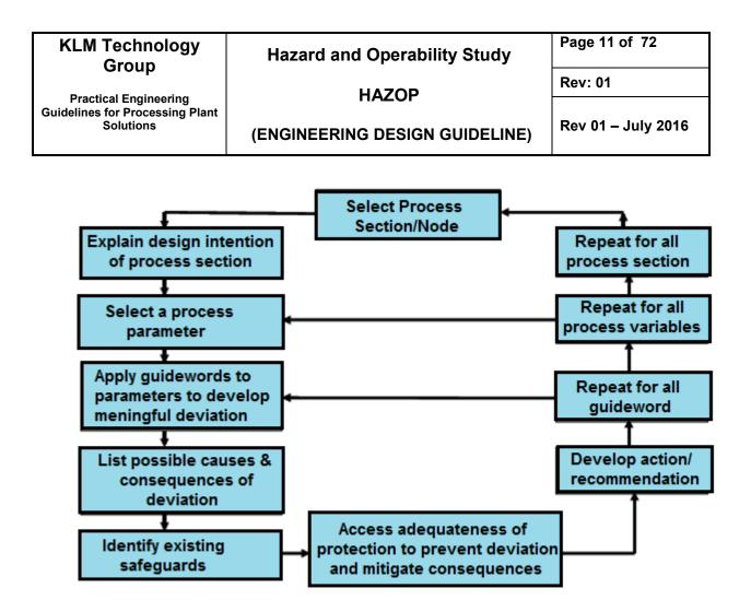
Figure 1: Typical HAZOP Procedure
