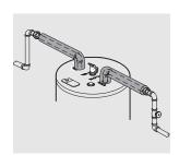
Typical horizontal piping arrangement
