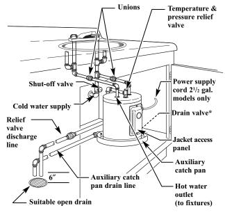
\*The drain valve is located below and to the right of jacket access panel and is not visible in this view.
