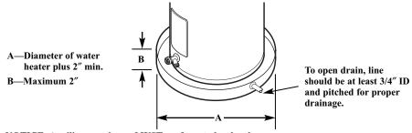
NOTICE: Auxiliary catch pan MUST conform to local codes. Catch Pan Kits are available from the store where the water heater was purchased, or any water heater distributor.
