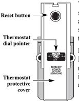
The illustration at the left shows the temperature adjustment dial used for setting the water temperature.
