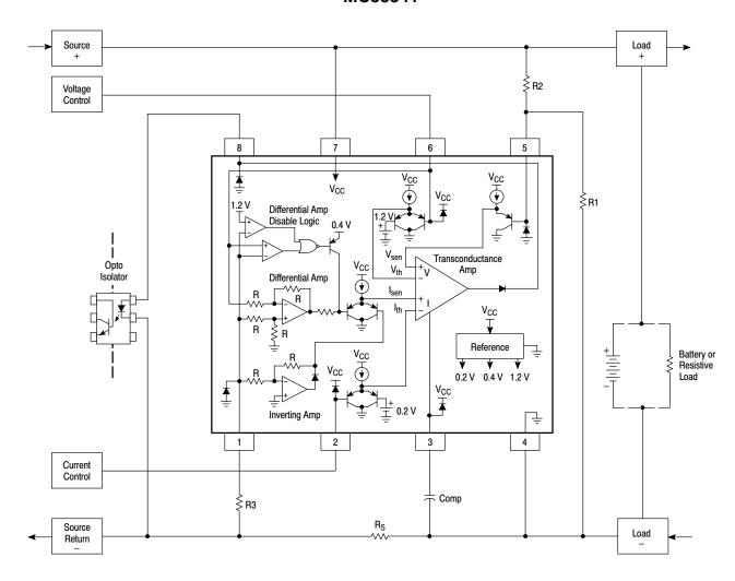
The above figure shows the MC33341 configured for source return low–side current sensing with externally adjustable voltage and current thresholds. Operation of this circuit is similar to that of Figure 15. The respective voltage and current regulation threshold can be adjusted over a range of 0 to 1.6 V and 0 V to 200 mV with respect to Pin 4.
