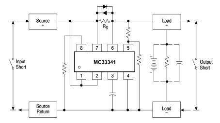
**NOTE:** An excessive load induced voltage across R<sub>S</sub> can occur if either the source input or load output is shorted. This voltage can easily be bounded with the addition of the diodes shown without degrading the current sensing accuracy. This bounding technique can be used in any of the MC33341 applications where high peak currents are anticipated.
