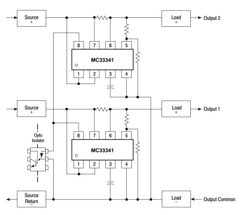
**NOTE:** Multiple outputs can be controlled by summing the error signal into a common optoisolator. The converter output with the largest voltage or current error will dominate control of the feedback loop.
