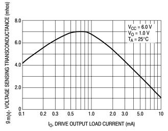
Figure 9. Transconductance Voltage Sensing Inputs to Drive Output
