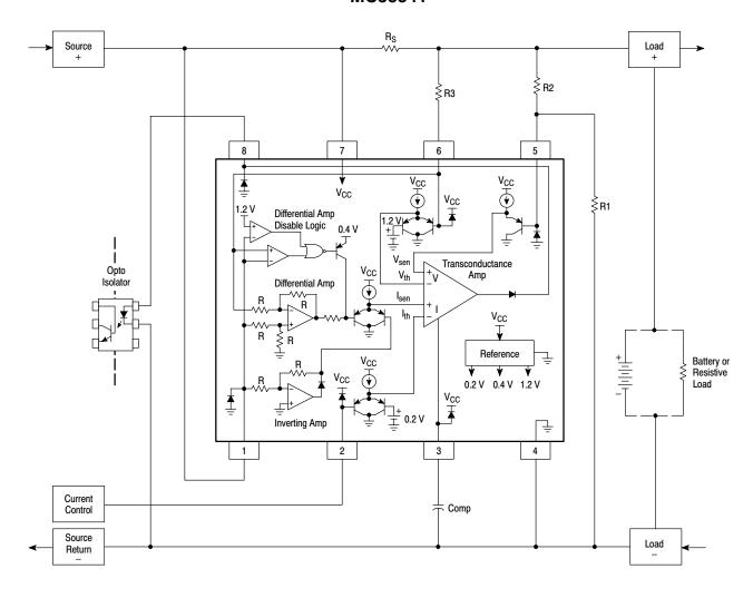
The above figure shows the MC33341 configured for source high–side current sensing with an externally adjustable current threshold. Operation of this circuit is similar to that of Figure 13. The current regulation threshold can be adjusted over a range of 0 V to 200 mV with respect to Pin 4.
