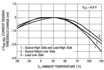
Figure 2. Current Sensing
