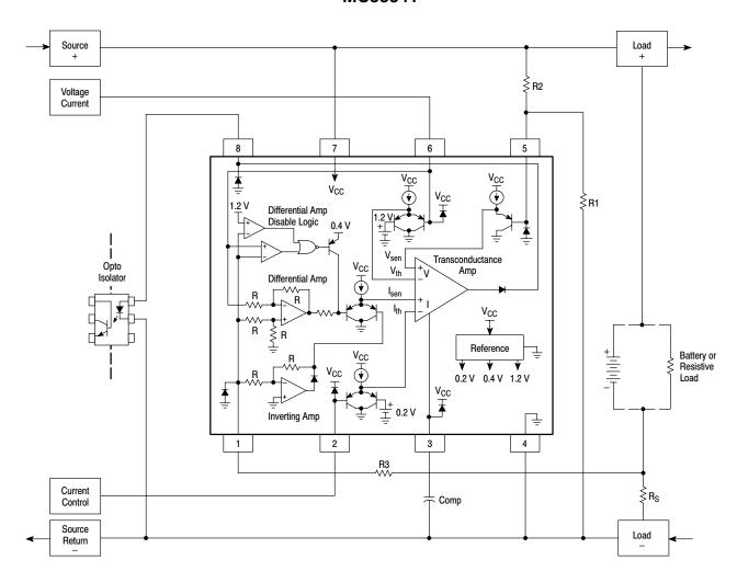
The above figure shows the MC33341 configured for load low–side current sensing with an externally adjustable voltage and current threshold. Operation of this circuit is similar to that of Figure 19. The respective voltage and current regulation threshold can be adjusted over a range of 0 to 1.2 V and 0 V to 200 mV, with respect to Pin 4.
