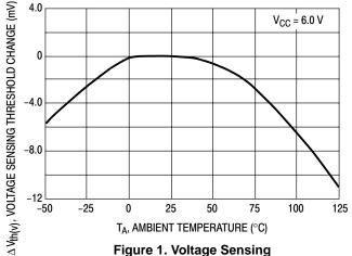
Figure 1. Voltage Sensing Threshold Change versus Temperature
