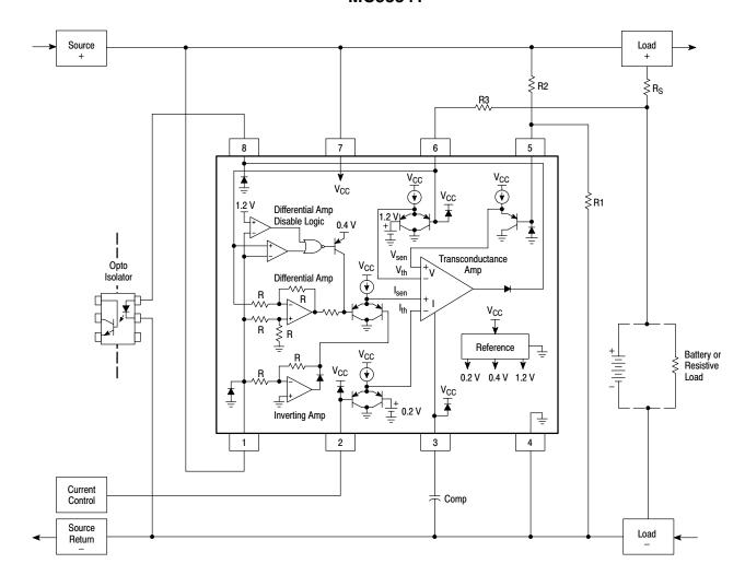
The above figure shows the MC33341 configured for load high–side current sensing with an externally adjustable current threshold. Operation of this circuit is similar to that of Figure 17. The current regulation threshold can be adjusted over a range of 0 V to 200 mV with respect to Pin 4.
