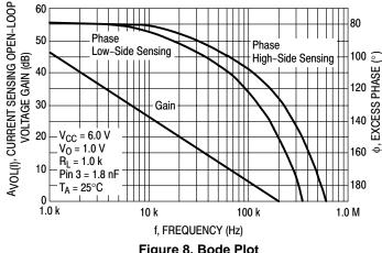
Figure 8. Bode Plot Current Sensing Inputs to Drive Output
