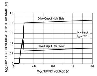
Figure 12. Supply Current versus Supply Voltage
