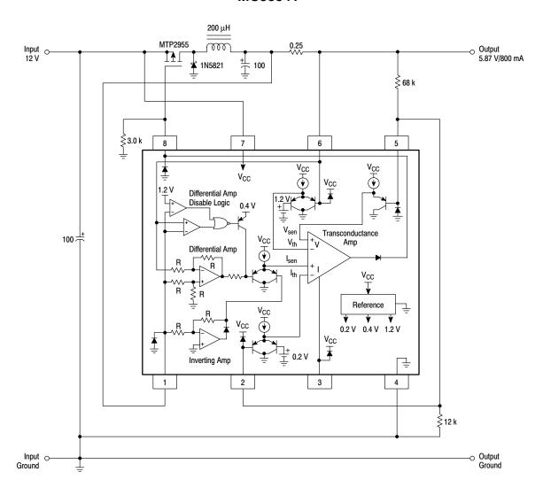
Figure 25 shows that the MC33341 can be configured as a high–side constant–current constant–voltage switch mode charger. This circuit operates as a step down converter. With a nominal input voltage and output load current as stated above, the switching frequency is approximately 28 kHz with and an associated conversion efficiency of 86 percent. The switching frequency will vary with changes in input voltage and load current.
