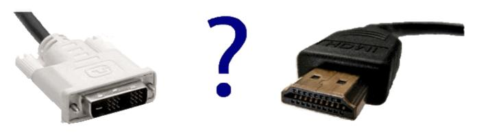
If your screen supports DVI (the first cable in the picture) move on to <u>Step 3A</u>, otherwise proceed to <u>Step 3B</u> if you will be using HDMI
