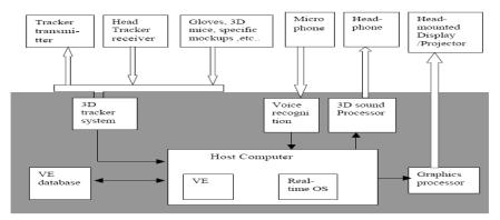
Figure. 2. Connectivity between elements of a Virtual Reality system
