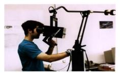
Figure. 4. BOOM (Binocular Omni-Orientation Monitor)
