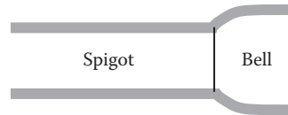
Figure 4.10 Bell-and-spigot ends of clay pipe sections.
