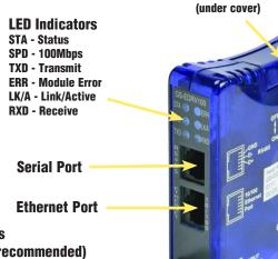
**Power Terminals** (Class 2 power recommended) Positive connection (+) or +10-36VDC Negative connection (-) or OVDC
