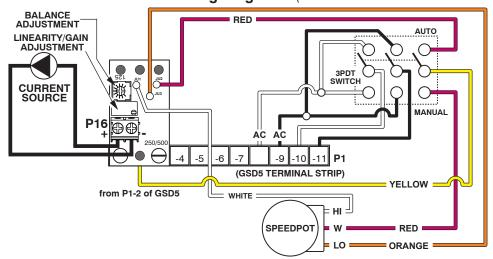
GSD5-240-10N4-V Basic Wiring Diagram – (refer to User Manual for more detailed wiring information)
