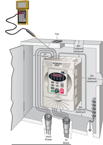
Warning: Maximum ambient temperatures must not exceed 50°C (122°F), or 40°C (104°F) for models 7.5 hp (5.5 kW) and higher!
