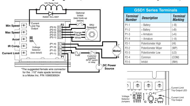
**GSD1-48-10N4X Basic Wiring Diagram** – (refer to User Manual for more detailed wiring information)
