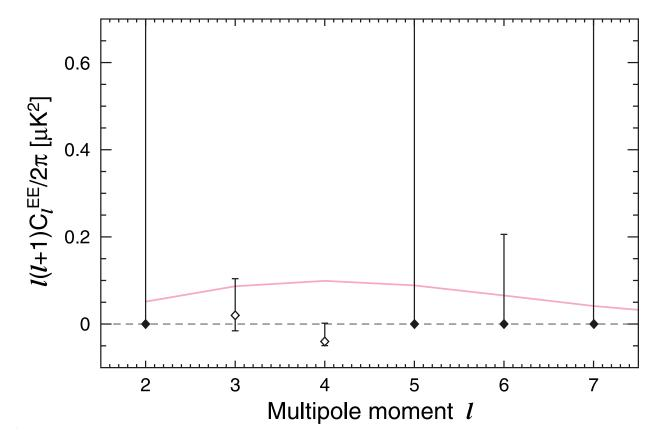
Fig. 10.— The EE power spectrum computed from the null sky maps,  $\frac{1}{2}S_{\text{Ka}} - \frac{1}{2}S_{\text{QV}}$ , where S = Q,U are the polarization Stokes parameters, and  $S_{\text{QV}}$  is the optimal combination of the Q and V band data. The pink curve is the best-fit theoretical spectrum from Dunkley et al. (2008). The spectrum derived from the null maps is consistent with zero.
