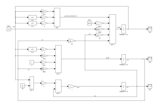
Figure 7.1: Simulink scheme of neuron model
