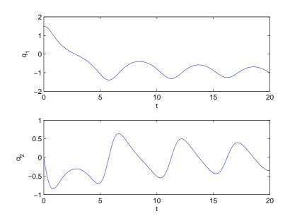
Figure 5.5: Time trajectory of Duffing equation
