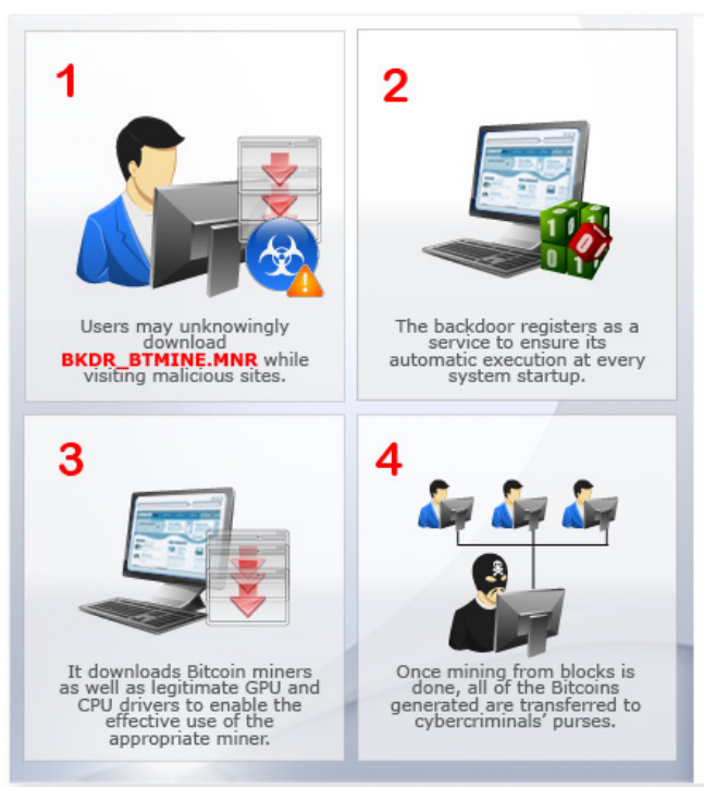
Figure 1. BKDR_BTMINER.MNR's infection diagram
