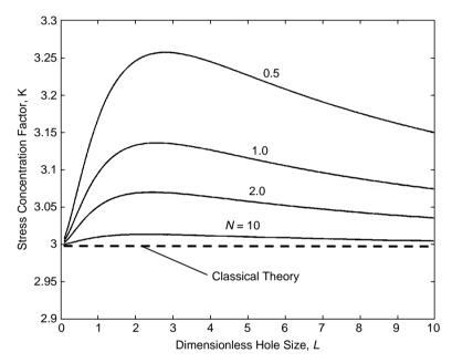
FIGURE 14-19 Stress concentration behavior for elastic material with voids.
