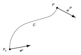
FIGURE 2-8 Continuity of displacements.
