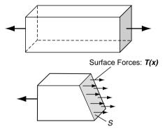
(b) Sectioned Axially Loaded Beam
