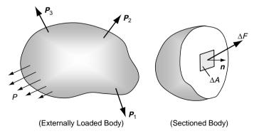
FIGURE 3-2 Sectioned solid under external loading.
