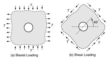
FIGURE 8-15 Stress-free hole under biaxial and shear loading.
