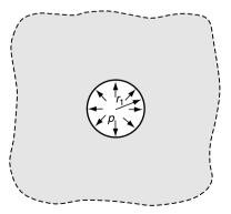
FIGURE 8-10 Pressurized hole in an infinite medium.
