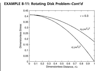
FIGURE 8-38 Stresses in a rotating disk.
