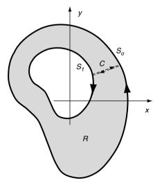
FIGURE 9-4 Multiply connected cross-section.
