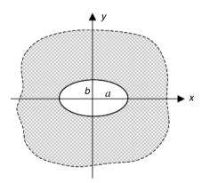
FIGURE 11-9 Elliptical hole in an infinite anisotropic plane.
