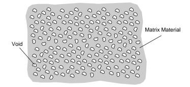
FIGURE 14-18 Elastic continuum with distributed voids.
