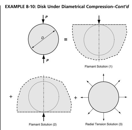
FIGURE 8-34 Disk under diametrical compression—superposition solution.
