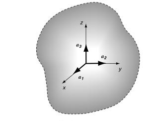
FIGURE 14-6 Unit concentrated loadings.
