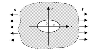
FIGURE 11-10 Infinite anisotropic plate with elliptical hole.
