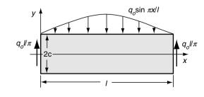
FIGURE 8-6 Beam carrying sinusoidal transverse loading.
