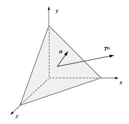
FIGURE 3-4 Traction on an oblique plane.
