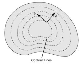
FIGURE 9-6 Contour lines for the torsion-membrane analogy.
