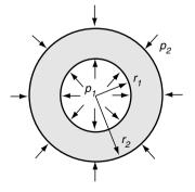
FIGURE 8-8 Thick-walled cylinder problem.
