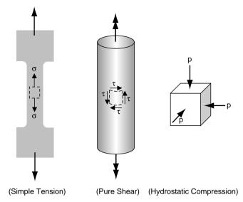
FIGURE 4-2 Special characterization states of stress.
