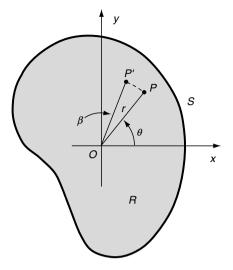
FIGURE 9-2 In-plane displacements for the torsion problem.
