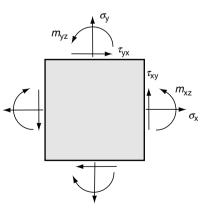
FIGURE 14-16 Couple stresses on planar element.
