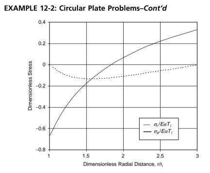
**FIGURE 12-4** *Stress distribution in annular plate*  $(r_o/r_i = 3)$ *.*
