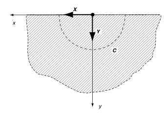
FIGURE 10-12 Concentrated force system on a half space.
