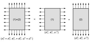
FIGURE 5-6 Two-dimensional superposition example.
