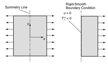
FIGURE 5-2 Line of symmetry boundary condition.
