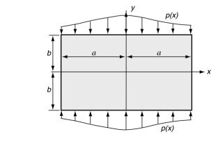
FIGURE 8-7 General boundary loading on a rectangular elastic plate.
