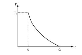
FIGURE 12-3 Temperature distribution in annular plate.
