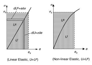
FIGURE 6-4 Strain and complementary energy for linear and nonlinear elastic materials.
