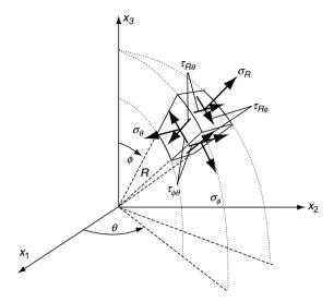
FIGURE 3-10 Stress components in spherical coordinates.
