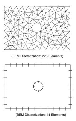
FIGURE 15-8 Comparison of typical FEM and BEM meshes.
