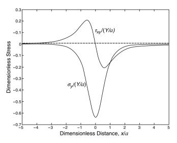
FIGURE 8-20 Normal and shear stress distributions below the free surface for the Flamant problem.
