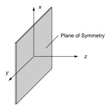
FIGURE 11-2 Plane of symmetry for a monoclinic material.
