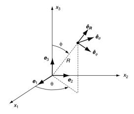
FIGURE 1-5 Spherical coordinate system.
