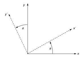
FIGURE 2-6 Two-dimensional rotational transformation.
