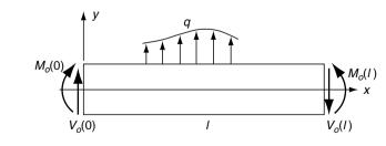
FIGURE 6-5 Euler-Bernoulli beam geometry.
