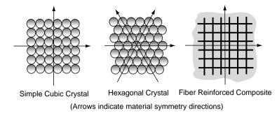
FIGURE 11-1 Material microstructures.
