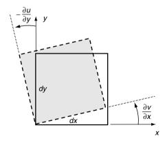
FIGURE 2-5 Two-dimensional rigid-body rotation.
