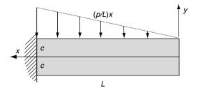
8-5. The cantilever beam shown in the figure is subjected to a distributed shear stress  $\tau_o x/l$  on the upper face. The following Airy stress function is proposed for this problem
