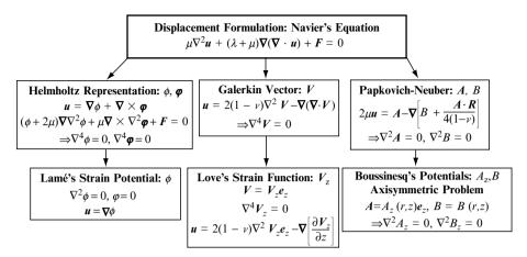
FIGURE 13-4 Displacement potential solutions.
