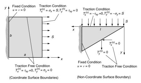
**FIGURE 5-4** *Example boundary conditions.*
