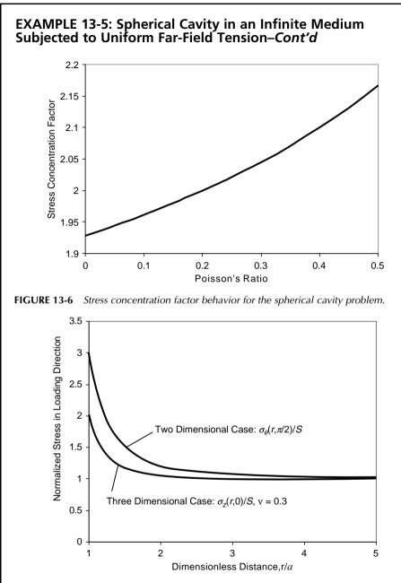
**FIGURE 13-7** Comparison of two- and three-dimensional stress concentrations around cavities.
