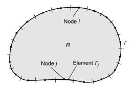
FIGURE 15-9 Boundary discretization using elements with constant approximation.
