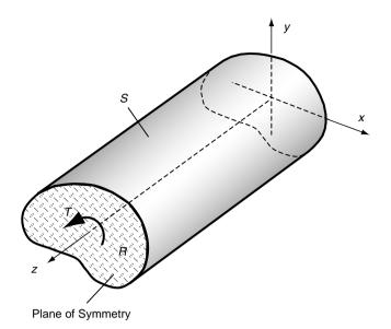
FIGURE 11-5 Torsion of an anisotropic bar.
