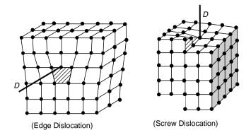
FIGURE 14-2 Schematics of edge and screw dislocations.
