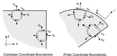
FIGURE 5-3 Boundary stress components on coordinate surfaces.
