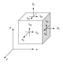
FIGURE 3-3 Components of the stress.
