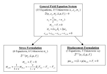
FIGURE 5-5 Schematic of elasticity field equations.
