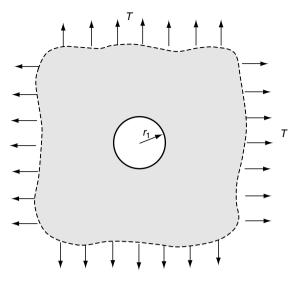
FIGURE 8-11 Stress-free hole under uniform biaxial far-field loading.
