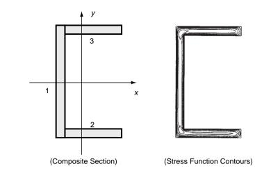
**FIGURE 9-14** Composite section of three thin rectangles.
