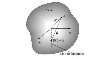
**FIGURE 14-11** *Line of dilatation along the negative x<sub>3</sub>-axis.*
