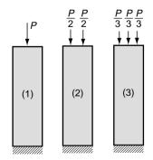
FIGURE 5-7 Statically equivalent loadings.
