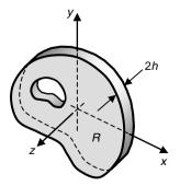
FIGURE 7-3 Thin elastic plate representing plane stress conditions.
