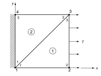
FIGURE 15-3 FEM analysis of elastic plate under uniform tension.
