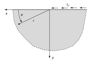
8-17. Show that the Flamant solution given by equations (8.4.31) and (8.4.32) can also be used to solve the more general wedge problem as shown.
