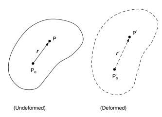
FIGURE 2-2 General deformation between two neighboring points.
