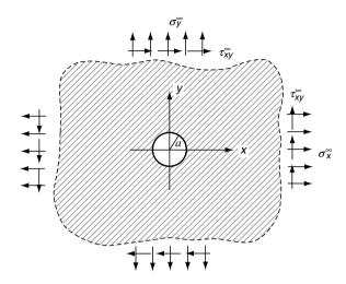
FIGURE 10-14 Stress-free hole under general far-field loading.
