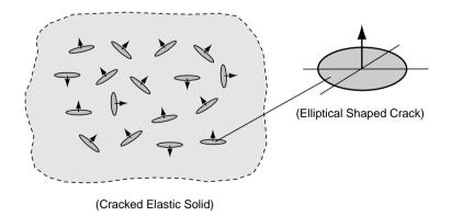
FIGURE 14-12 Elastic solid containing a distribution of cracks.
