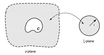
FIGURE 10-15 General mapping for infinite plane with interior hole.
