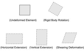
FIGURE 2-3 Typical deformations of a rectangular element.
