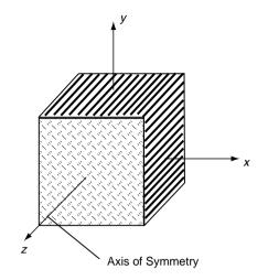
FIGURE 11-4 Axis of symmetry for a transversely isotropic material.
