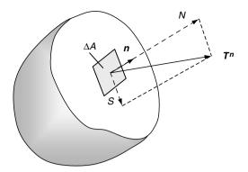
FIGURE 3-6 Traction vector decomposition.
