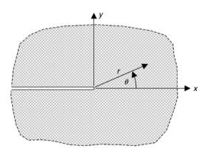
FIGURE 11-11 Crack in an infinite anisotropic plane.
