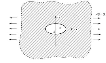
FIGURE 10-17 Infinite plane with an elliptical hole.
