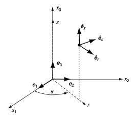
FIGURE 1-4 Cylindrical coordinate system.
