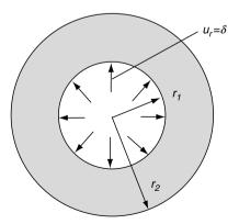
8-12. A long composite cylinder is subjected to the external pressure loading as shown. Assuming idealized perfect bonding between the two materials, the normal stress and displacement will be continuous across the interface  $r = r_1$ . Under these conditions, determine the stress and displacement fields in each material.
