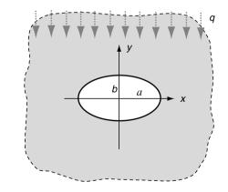
**FIGURE 12-6** Flow of heat around an elliptical hole in an infinite plane.
