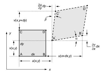
FIGURE 2-4 Two-dimensional geometric strain deformation.
