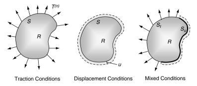
FIGURE 5-1 Typical boundary conditions.
