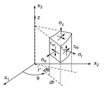
FIGURE 3-9 Stress components in cylindrical coordinates.
