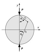
FIGURE 8-35 Disk under diametrical compression.
