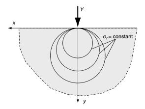
FIGURE 8-21 Radial stress contours for the Flamant problem.
