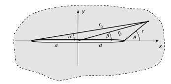
FIGURE 10-20 Crack geometry.
