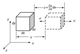
FIGURE 6-1 Deformation under uniform uniaxial stress.
