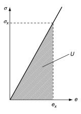
FIGURE 6-2 Strain energy for uniaxial deformation.
