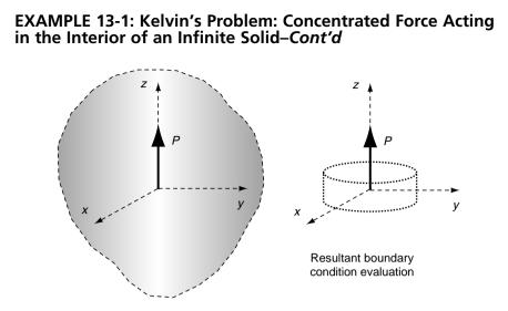
FIGURE 13-1 Kelvin's problem: concentrated force in an infinite medium.
