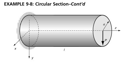
**FIGURE 9-20** Flexure of a beam of circular section.
