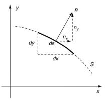
FIGURE 9-3 Differential surface element.
