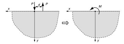
FIGURE 8-23 Half space with concentrated surface moment loading.
