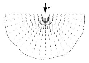
FIGURE 8-22 Displacement field for Flamant problem.
