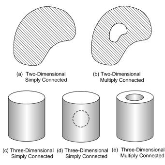
FIGURE 2-9 Examples of domain connectivity.
