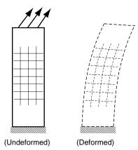
FIGURE 2-1 Two-dimensional deformation example.
