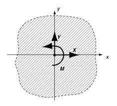
FIGURE 10-11 Concentrated force system in an infinite medium.
