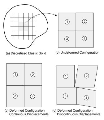
FIGURE 2-7 Physical interpretation of strain compatibility.
