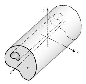
FIGURE 7-1 Long cylindrical body representing plane strain conditions.
