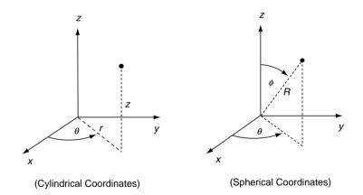
FIGURE A-1 Cylindrical and spherical coordinate systems.
