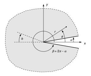
FIGURE 8-29 Crack problem geometry.
