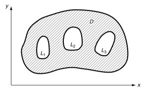
FIGURE 10-3 Multiply connected domain.
