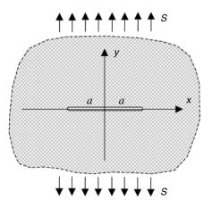
FIGURE 11-12 Central crack in an infinite anisotropic plane.
