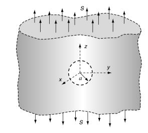
FIGURE 13-5 Spherical cavity in an infinite medium under tension.
