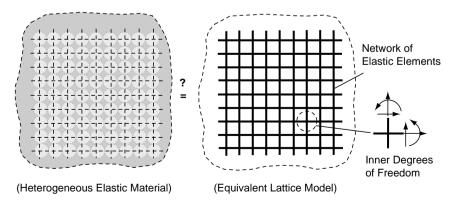
FIGURE 14-15 Heterogeneous materials with microstructure.
