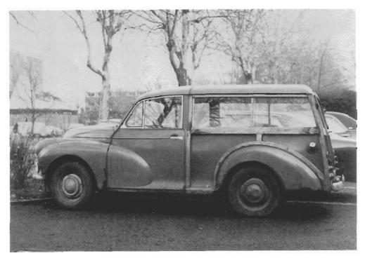
Fig. 27.3. The Morris Traveller – a classic of the 1950s with wooden members used as an integral part of the monocoque body shell.
