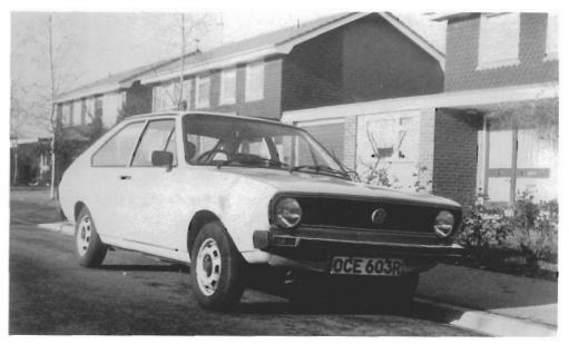
Fig. 27.2. The Volkswagen Passat – a typical 1970s pressed-steel body with no separate chassis. For a given material this 'monocoque' construction gives a minimum weight-to-strength ratio.
