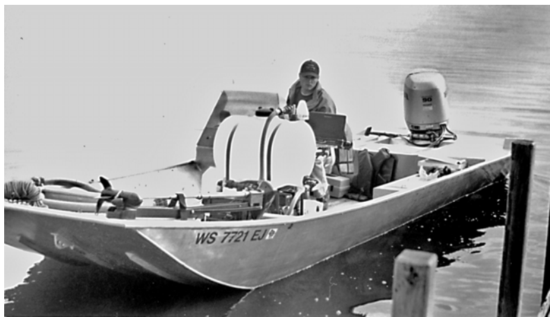
FIGURE 16.4 Typical herbicide application equipment. Notice the GPS antennae and the on-board computer.
