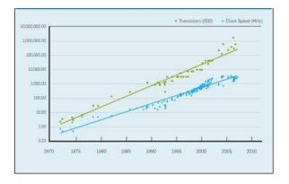
In this case of going from 8086 to i7, the speed goes up by 880 times during this period, doubled every 44 months.
