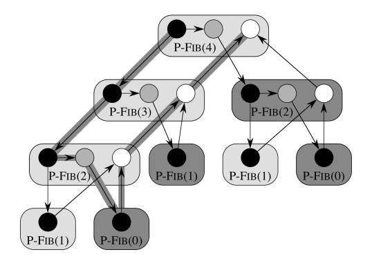
Take the top node for example, to calculate Fib(4), a process does three things: it spawns a black node (Line 3) to calculate Fib(3), and at the same time, proceeds (Line 4), via a grey node, to find out Fib(2), then wait for their completion (Line 5), and finally reports the result in a white node (Line 6).
