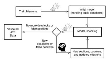
Fig. 7. The ATS configuration data validation process
