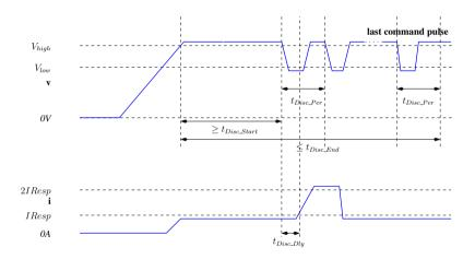
Fig. 7. Graphical specification of DSI3 discovery mode requirements
