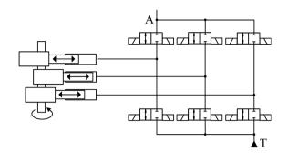
Fig. 1. The hydraulic architecture of a digital pump-motor. The figure shows three pistons connected to a rotating shaft to the left. Each piston is connected via valves to a high pressure line A and a tank line T.
