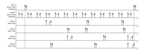
Fig. 6. Example of resulting real-time schedule for three cylinders. Dashed lines denote limits of period of the shaft, up arrows denotes release time, down arrows denote completion time.
