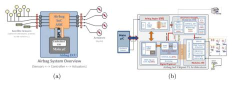
**Fig. 4.** A typical airbag system: (a) overview; (b) airbag SoC chipset top-level implementation architecture
