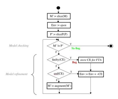
Fig. 2. CEGAR-like verification loop
