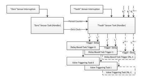
Fig. 3. The proposed architecture of the software of the DHPMS
