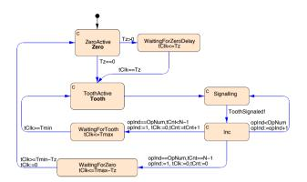
Fig. 4. The timed automaton describing triggering of zero sensor and tooth sensor handling tasks
