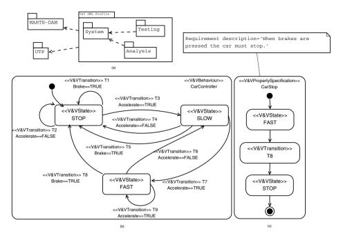
**Fig. 1.** Overview of V&V UML Profile: top-level packages (V&V UML Profile) (a), model of a car controller (b), property specification (c)
