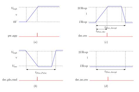
**Fig. 6.** Graphical specification of events of interest: (a) power applied; (b) discoverly pulse command; (c) sensor response; and (d) sensor no response
