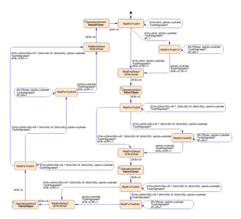
Fig. 5. The automaton describing triggering of valve tasks
