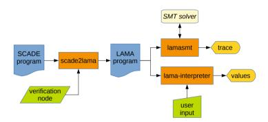
Fig. 6. Framework components and their interaction
