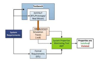
Fig. 1. Assertion-based monitoring flow with STL assertion language and AMT tool
