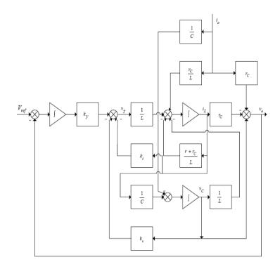
Fig. 6. Steady-State Error Model of PWM push-pull dc-dc converters
