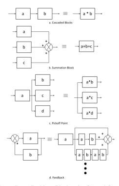
Fig. 3. Basic Building Blocks of a Control System
