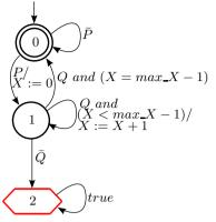
Fig. 1. Example of the BTC pattern modeling the process to close the gate after a train approaches. The parameter of the pattern are as follows:
