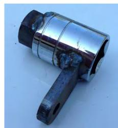
In the Switch Stand box install the socket with its wing in the clevis fork with a clevis pin and cotter pin.
