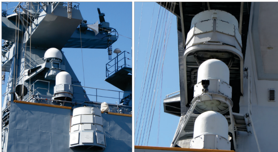
Figure 24 & 25: The EW TK-25 system on board the Grigorovich class frigate Admiral Makarov (left) and another configuration of the same system on board the Steregushchii class corvette Stoiki (right).
