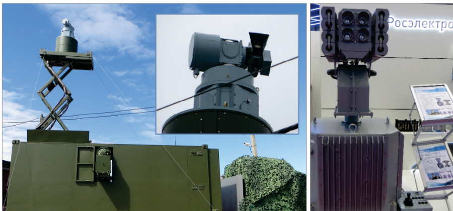
Figure 26 & 27: The MDM-2 laser jamming system (left) and the Grach dazzling system (right).
