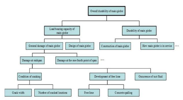
Fig. 2. Part of the process of evaluating overall durability of main girder
