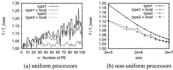
Figure 6: Evaluation of Partitioning Algorithms
