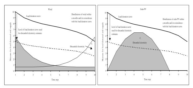
Figure 7: Illustrative representation of the contribution of the wind and solar PV power supply within the 10 time steps of a month: their coincidence with the Load Duration Curve and the method to calculate the amount of discarded wind and solar PV electricity.
