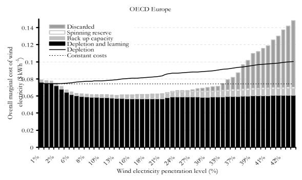
Figure 11b: The marginal cost development of wind electricity in OECD Europe with increasing wind electricity penetration subdivided in different cost components (Experiment A).
