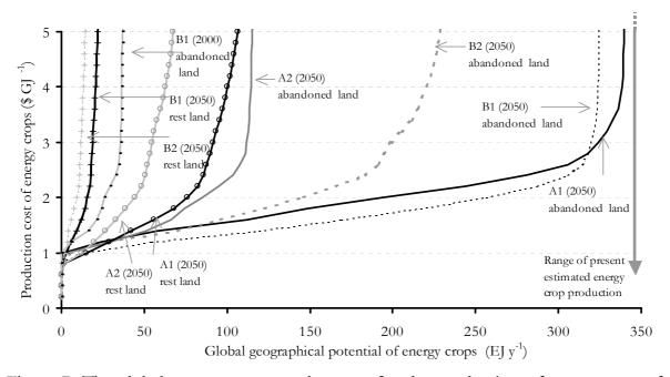
Figure 7: The global average cost-supply curve for the production of energy crops for four SRES scenarios for the year 2050 and the cost-supply curve at abandoned agricultural land for the year 2000 for the B1 scenario is also shown.
