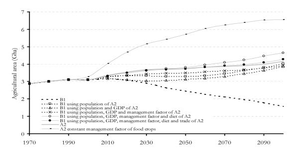
Figure 14: The global agricultural land area over time for several scenarios that convert the B1 scenario to A2 in various steps, as simulated by the IMAGE 2.2 model.
