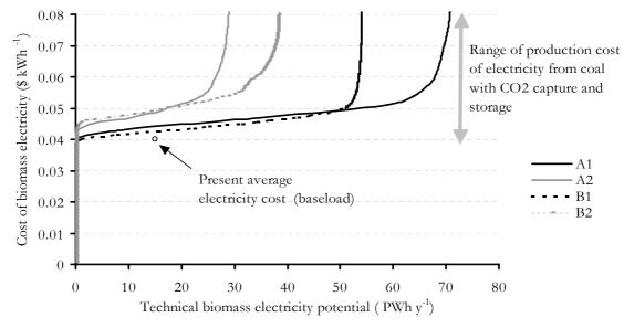
Figure 11: The cost-supply curve for the year 2050 of electricity using BIGCC conversion technology using energy crop produced at abandoned agricultural land and rest land as feedstock for the four SRES scenarios compared to present average baseload electricity production costs and estimates of future electricity production cost from coal-fired plants with CO<sub>2</sub> capture and storage.
