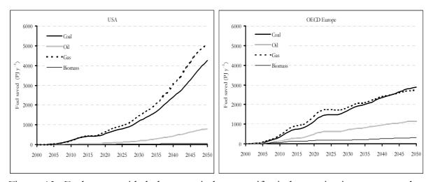
Figure 13: Fuel use avoided due to wind power if wind capacity increases to about 38%(USA) - 43% (OECD Europe) penetration in 2050 in Experiment B.
