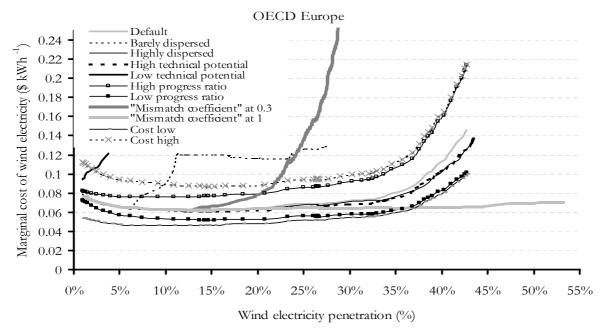
Figure 16: Sensitivity analysis for four parameters influencing the electricity penetration and cost of wind electricity if wind capacity increases in the USA and OECD Europe from the year 2000 to 2050 (Experiment B).
