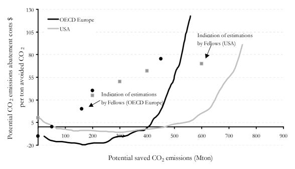
Figure 14: The potential CO<sub>2</sub> abatement cost for wind electricity with increasing wind power penetration (Experiment B). For comparison, also results of Fellows (2000) are shown.
