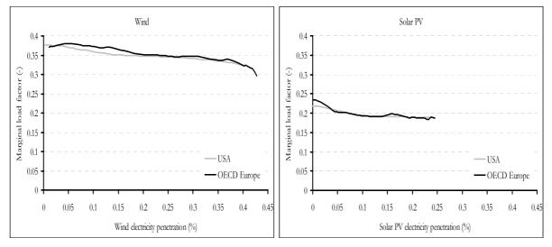
Figure 8: Marginal load factor with increasing electricity<sup>55</sup> penetration of wind and solar PV<sup>56</sup>
