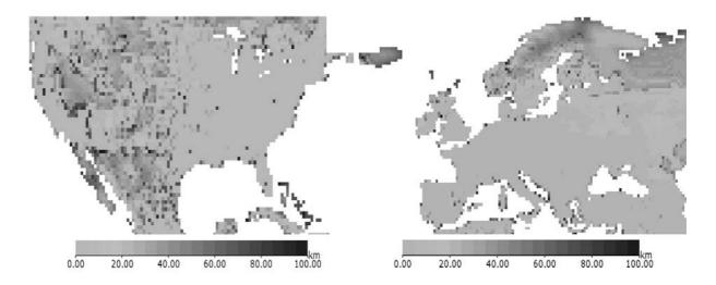
Figure 3: Spatial distribution of the estimated transmission distances at grid cell level in USA and OECD Europe. A distance of e.g. 40 km means that within a radius of 40 km from that grid cell, an average power demand is found equal to 50 MW.
