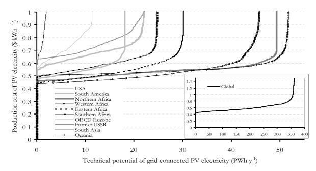
Figure 8: Cost-supply curve for grid-connected centralised PV applications, globally, and for ten regions (present situation). The black square in the 'global' curve indicates the present electricity consumption and range of production costs of electricity (Goldemberg, 2000).
