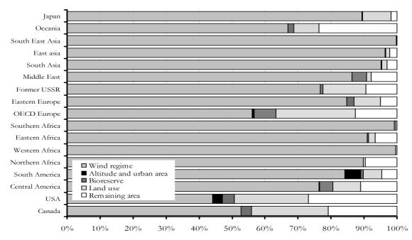
Figure 3: The regional siting constraints for the installation of wind turbines. In this figure, the remaining category equals the suitability factor,  $f_i$ .
