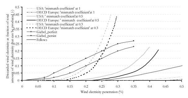
Figure 9: Average value of discarded wind electricity in the USA and OECD Europe indicated as fraction of the potentially produced wind electricity, as function of the penetration (on electricity basis), within Experiment A and for three values of the 'mismatch coefficient'  $\varphi$ .
