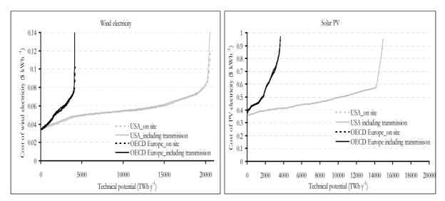
Figure 4: The cost supply curve of wind and solar PV electricity in the year 2000 for USA and OECD Europe with and without inclusion of transmission costs.
