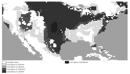
Figure 8a: The areas in the USA where wind electricity can be generated at costs below 0.25, 0.15, 0.10 and 0.06 \$ kWh<sup>-1</sup>
