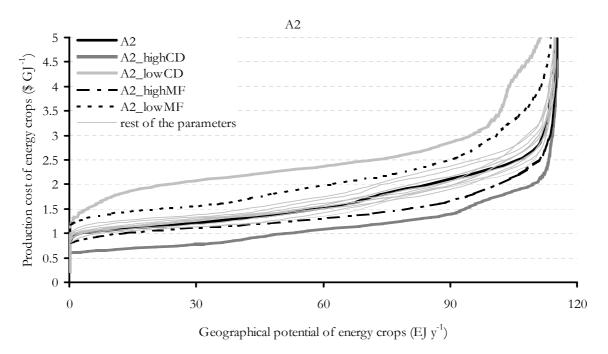
Figure 12b: Sensitivity analysis of the cost-supply curve of energy crops at abandoned agricultural land for the year 2050 within the A2 scenario by varying most important input parameters with  $\pm$  25%. The progress ratio has been varied between 0.85 and 0.99.
