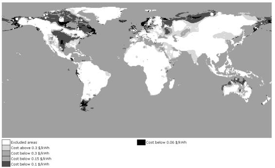
Figure 7: The areas where wind electricity can be generated at various cost classes (costs below 0.20, 0.15, 0.10 and 0.05 \$ kWh<sup>-1</sup>).
