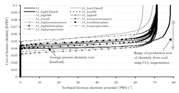
Figure 12c: Sensitivity analysis of the cost-supply curve of biomass electricity for the year 2050 for the A1 scenario by varying most important input parameters with  $\pm$  25%. (In the legend, *CD* means substitution elasticity, *MF* means management factor, *eff* means conversion efficiency.)
