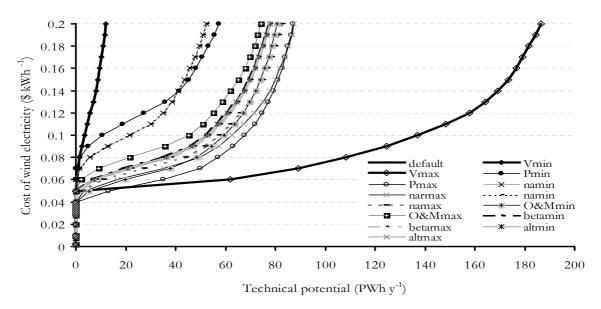
Figure 11: Sensitivity of input parameters ( $\eta_{ar}$ ,  $\eta_a$ ,  $w_i$ , Pr,  $\varepsilon$ ,  $\beta$  and  $V_{10}$ ,) on the global cost-supply curve
