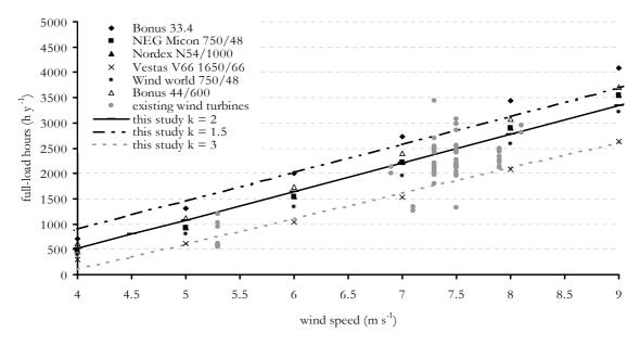
Figure 5: The full-load hours as a function of the average annual wind speed for a set of seven commercially available turbines operating at various average wind speeds and Weibull factors (k = 1.5; k = 2.0 (default); k = 3.0). Wind turbine output data of 7 wind farms are included for comparison.
