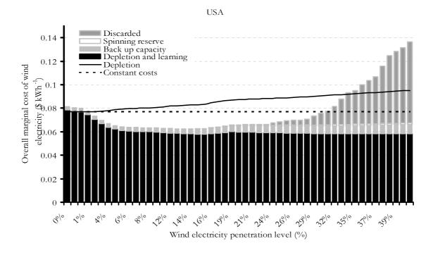
Figure 11a: The marginal cost development of wind electricity in the USA with increasing wind electricity penetration subdivided in different cost components (Experiment A).
