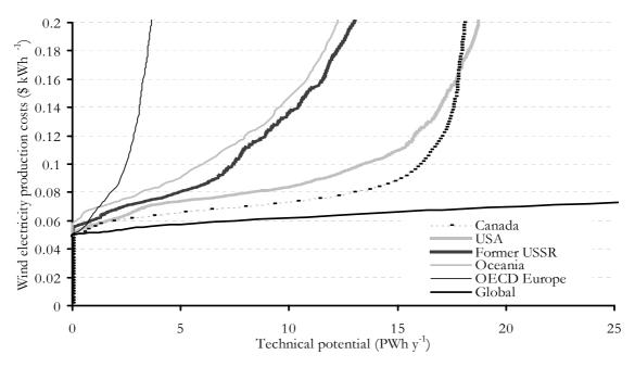
Figure 9: Regional cost supply curve for wind energy (\$ kWh<sup>-1</sup> versus PWh y<sup>-1</sup>) for D = 4 MW km<sup>-2</sup>. For comparison the global cumulative curve is also presented.
