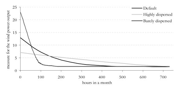
Figure 15: Assumptions regarding the monthly Load Supply Curve of wind power resulting from the assumed geographical dispersion, as used in the sensitivity analysis.
