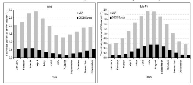
Figure 1: Monthly variation in an average year of the technical potential of wind and solar PV electricity at cut off on site costs of 2 \$ kWh-1, for USA and OECD Europe as constructed from Chapter 5 and 6 and used in the simulation experiments.
