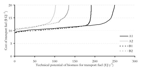
Figure 10: The cost supply curve for the year 2050 of biomass liquid fuel (synthetic FT diesel) using energy crop produced at abandoned agricultural land and rest land as feedstock for the four SRES scenarios
