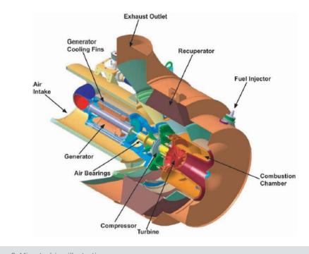
Figure 2. Microturbine illustration. Graphic credit Capstone Turbine Corporation.
