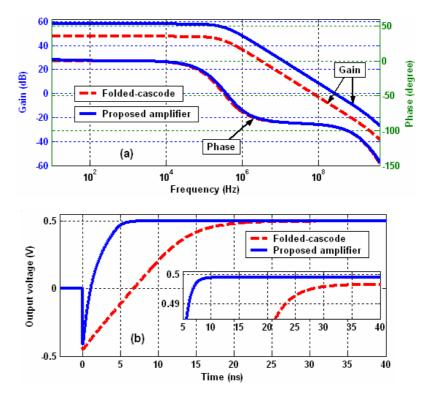
**Fig. 2.** (a) Open loop small-signal frequency response, and (b) settling response.
