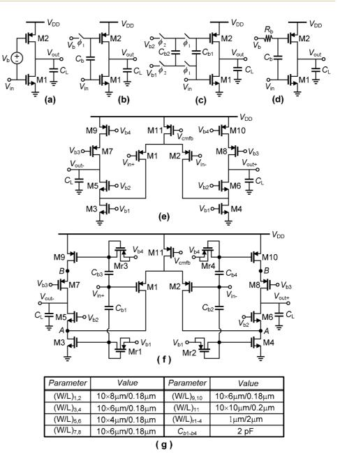
Fig. 1. (a) General structure of a class AB output stage, implementation of class AB output stage by (b) a switch and capacitor, (c) dynamic level shifting, (d) a large resistor and capacitor, (e) conventional class A folded-cascode amplifier, (f) proposed class AB folded-cascode amplifier, and (g) simulated device parameters.
