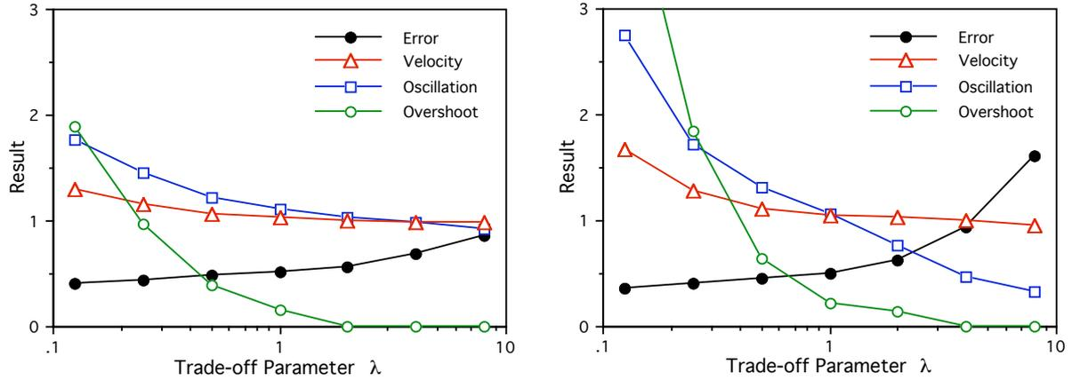
Figure 4: Varying levels of learned performance for the control system of Figure 1: with error plus integrated velocity  $\lambda\Phi_{vel}$  minimized (left) and error plus oscillations  $\lambda\Phi_{osc}$  minimized (right).
