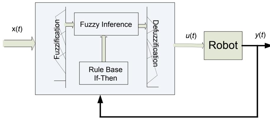
Figure 5: Block diagram for a fuzzy robot controller.
