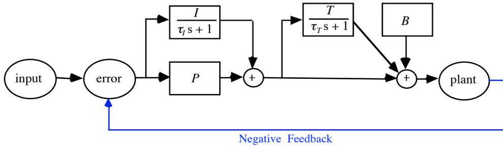
Figure 1: Simplified control system with parameters  $\{I, P, T, B\}$  to be learned using a gradient descent algorithm.
