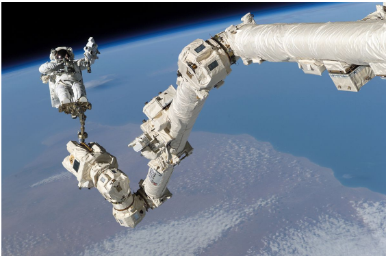
The Canadarm2 robotic manipulator on the International Space Station is operated by controlling the angles of its joints. Calculating the final position of the astronaut at the end of the arm requires repeated use of trigonometric functions of those angles.
