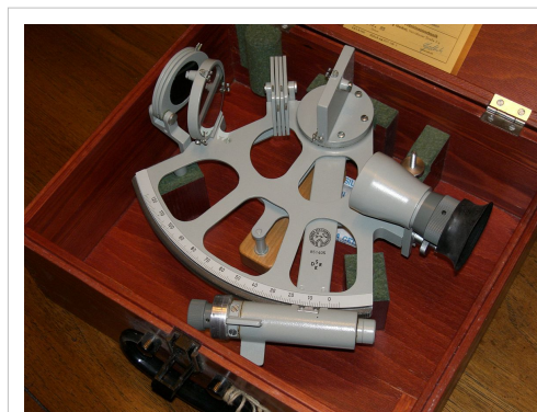
Sextants are used to measure the angle of the sun or stars with respect to the horizon. Using trigonometry and a marine chronometer, the position of the ship can be determined from such measurements.
