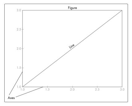
Figure 6-1: Architecture of a matplotlib plot
