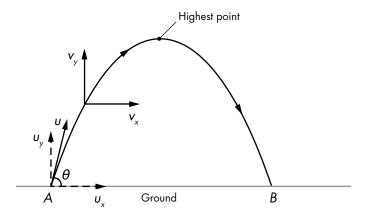
Figure 2-13: Motion of a ball that's thrown at point A—at an angle (θ) with a velocity (υ)—and that hits the ground at point B
