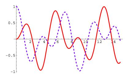
The motion is a combination of oscillations at the two normal mode frequencies.
