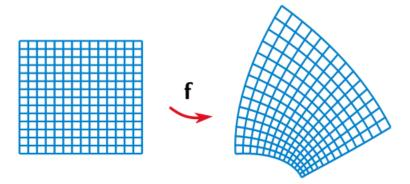
Figure 63: **f** is a conformal map because it preserves the angles of intersection of all lines. However, the distance between the lines, and therefore the angles between them away from their points of intersection, are not preserved in a conformal transformation. This figure is taken from Wikipedia.
