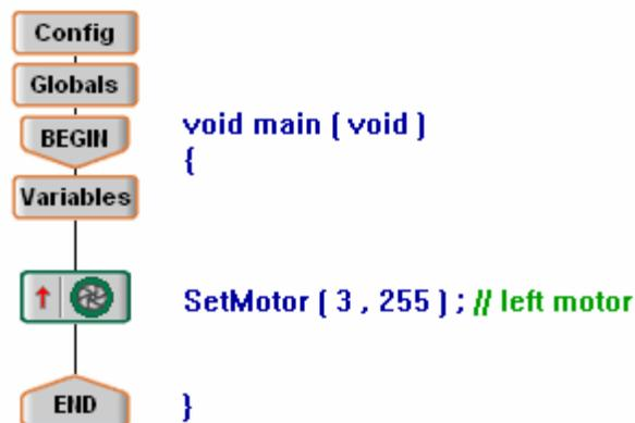
7. In the similar way drag and drop one more motor module to configure the right motor. Assume right motor is connected to motor port 2 and it is set to counter-clockwise direction.
