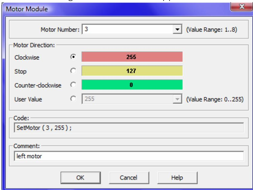
“**Motor Number**” is the motor port number to which the motor is connected to. Here left motor is assumed to be connected to port 3. So 3 is selected.
