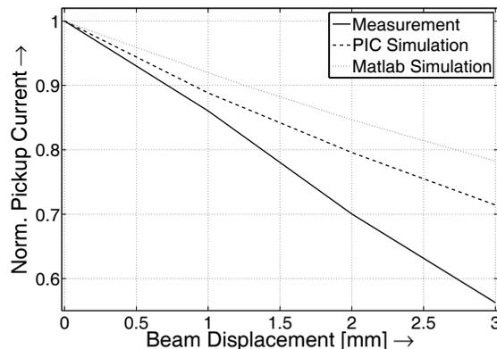
Figure 5: Simulation and measurement results on 6 GHz beam harmonic as a function of beam displacement. “0 mm” refers to the initial distance of the probe to the beam center (15 mm). The plots have been normalized to the respective currents at the initial position.
