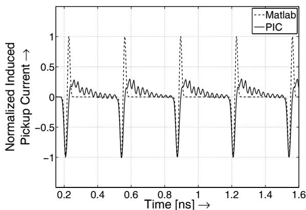
Figure 2: Comparison of pickup current signals in time domain gathered with Matlab analysis (dashed) and PIC code (solid) for a circular pickup with diameter  $d=3$  mm and a 6 MeV electron beam. The curves have been normalized to the maximum induced current obtained by the Matlab calculation.
