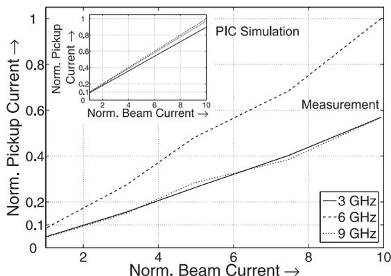
Figure 4: Comparison of PIC simulation and measurement concerning pickup current versus beam current. Both simulation and measurement data are normalized to the maximum occurring pickup current showing nearly the same linear dependence in the plot.
