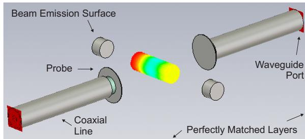
Figure 1: 3D model of CST PS simulation setup showing two opposite circular pickups as well as emission surfaces for the beam.
