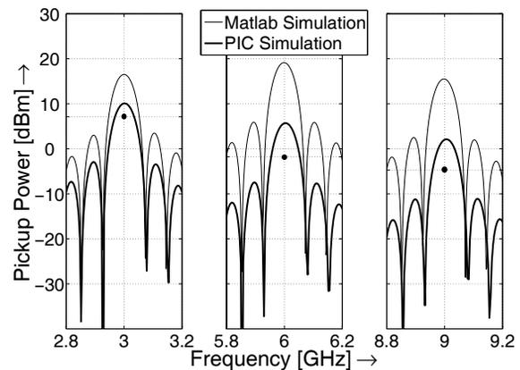
Figure 3: Comparison of spectral power distribution between Matlab simulation (fine), PIC simulation (bold) and measurement (dots). Despite beam spreading, the measured values are in close vicinity to the simulation results.
