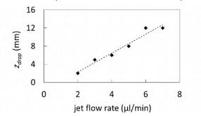
Figure 3. Position of microdroplet formation in terms of jet flow rate
