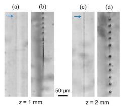
Figure 2. Effect of DVB concentration on droplet formation inside the channel. (a) and (c) correspond to 0.5 wt% DVB and 95.5 wt% ethanol, (b) and (d) to 10 wt% DVB and 90 wt% ethanol. The flow direction is upward. Arrows indicate the grey lines which show nanodroplets in the case of 0.5 wt% DVB
