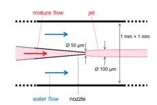
Figure 1. Flow configuration of the 3D co-flow microfluidic jet
