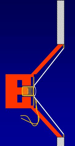
Baffle prevents front-back interaction: improved low frequency performance
