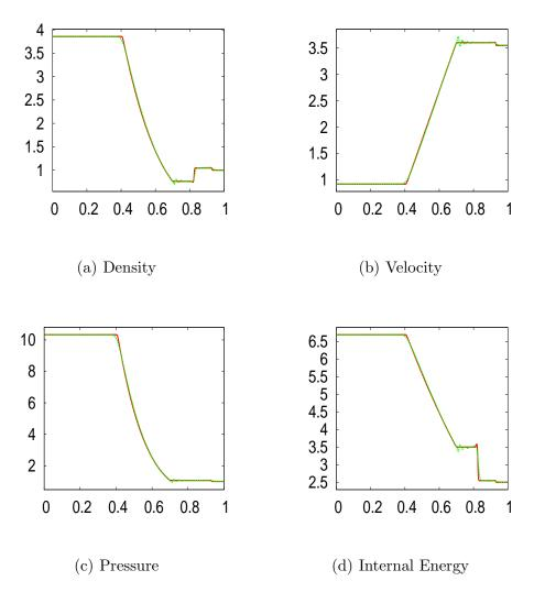
Fig. 8. Numerical results of the Mach 3 shock tube problem at t = .09s. The explicit baseline solution is plotted in red, and the solution from our method is plotted in dotted green.
