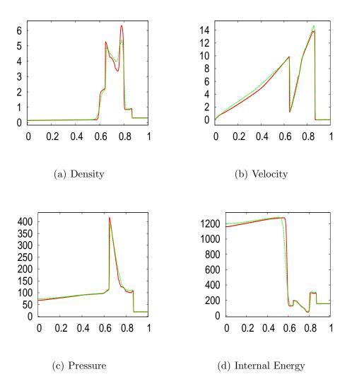
Fig. 10. Numerical results of the interacting blasts shock tube problem at t = .038s. The explicit baseline solution is plotted in red, and the solution from our method is plotted in dotted green.
