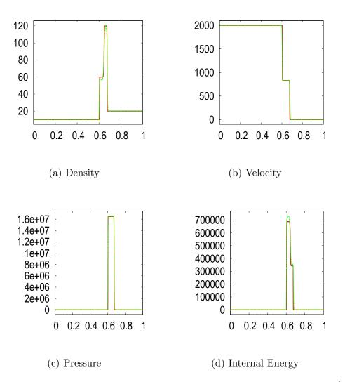
Fig. 9. Numerical results of the High Mach shock tube problem at  $t = 1.75 \times 10^{-4} s$ . The explicit baseline solution is plotted in red, and the solution from our method is plotted in dotted green.
