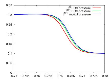
Fig. 2. A blow-up of the pressure plot for example 6.1.1 at time t(n) = .149s and t(n + 1) = .15s, showing that the implicit pressure calculated in equation (14) is a good approximation to what the pressure will be at time  $t^{n+1}$  emphasizing the implicit nature of our scheme.  $p^n$  is also plotted to emphasize the difference between using an implicit and explicit pressure.
