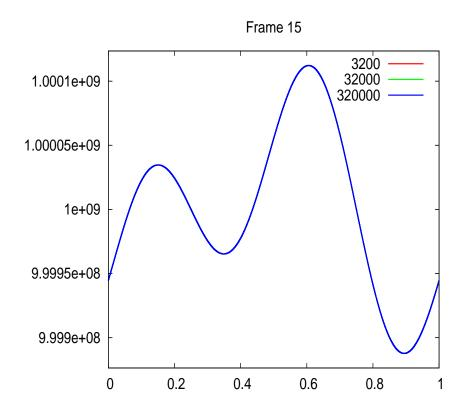
Fig. 13. Numerical results showing pressure in the smooth flow test at 3200, 32000 and 320000 grid cells. We used an effective sound speed based CFL number of 3, 30 and 300 respectively at  $t = 1.5 \times 10^{-5} s$ . Since  $\Delta t$  stays constant, the solution remains relatively unchanged even as we get huge time step gains.
