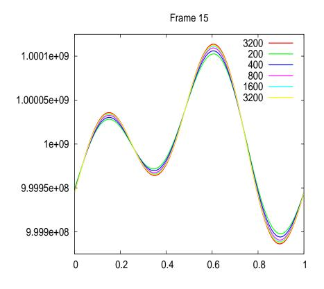
Fig. 12. Numerical results comparing the pressure in smooth flow test at 200, 400, 800, 1600, and 3200 grid cells with an effective sound speed based CFL number 3 at  $t = 1.5 \times 10^{-5} s$ . The red curve is the explicit simulation run at 3200 grid cells with a CFL number .5.
