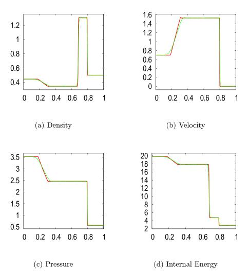
Fig. 6. Numerical results of the Lax's shock tube problem at t = .12s. The explicit baseline solution is plotted in red, and the solution from our method is plotted in dotted green.
