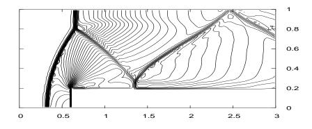
Fig. 14. Numerical results showing the contour plots of density for the flow past a step test on a grid of size 120x40 at t = 4s. 30 contours are plotted in the range [.2568, 6.067].
