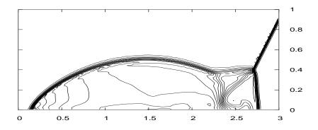
Fig. 15. Numerical results showing the contour plots of density for the double mach reflection of a strong shock on a grid of size 240x60 at t = .2s. 30 contours are plotted within the range [1.731, 20.92].
