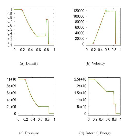
Fig. 7. Numerical results of the strong shock tube problem at  $t = 2.5 \times 10^{-6} s$ . The explicit baseline solution is plotted in red, and the solution from our method is plotted in dotted green.
