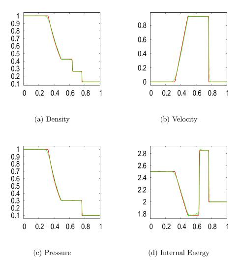
Fig. 5. Numerical results of the Sod shock tube problem at t = .15s. The explicit baseline solution is plotted in red, and the solution from our method is plotted in dotted green.
