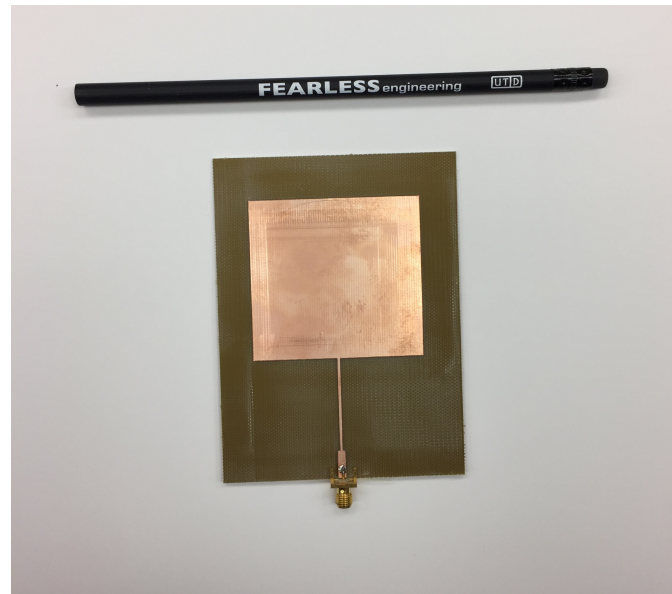
Figure 4.19. Fabricated patch antenna
