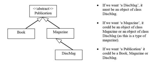
In other words we can 'substitute' an object of any subclass where an object of a superclass is required. This is NOT true in reverse!
