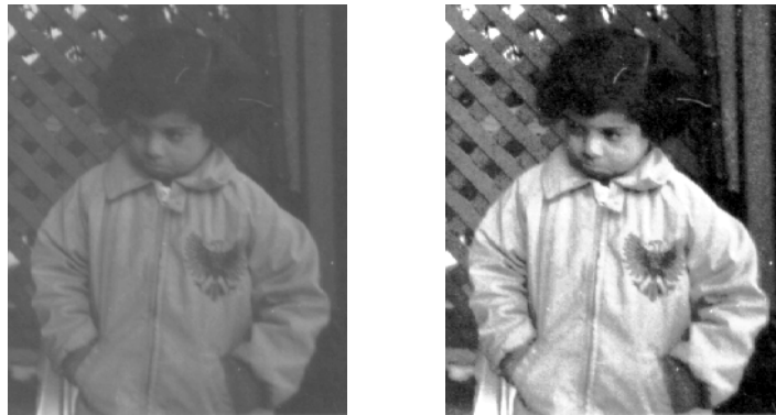
Figure 10-10: Pout.tif Before and After Histogram Equalization
