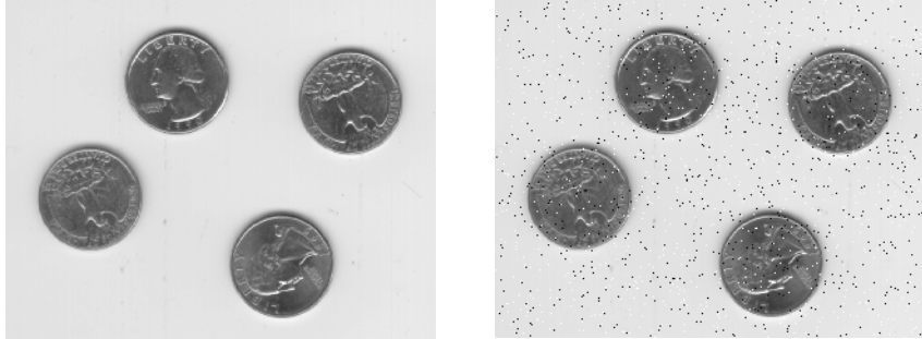
Figure 10-12: Eight.tif Before and After Adding Salt-and-Pepper Noise
