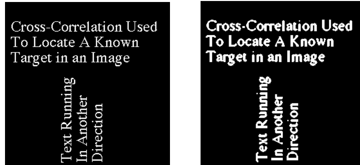
Figure 9-10: Text.tif Before and After Applying a Lookup Table Operation
