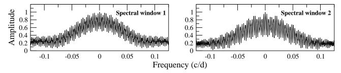
Fig. 3. Spectral windows showing the difference in aliasing between Set 1 and Set 2
