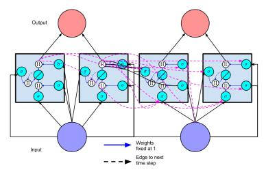
Figure 11: A recurrent neural network with a hidden layer consisting of two memory cells. The network is shown unfolded across two time steps.
