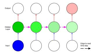
Figure 8: A visualization of the vanishing gradient problem, using the network depicted in Figure 7, adapted from Graves [2012]. If the weight along the recurrent edge is less than one, the contribution of the input at the first time step to the output at the final time step will decrease exponentially fast as a function of the length of the time interval in between.
