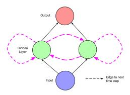
Figure 3: A simple recurrent network. At each time step t, activation is passed along solid edges as in a feedforward network. Dashed edges connect a source node at each time t to a target node at each following time t+1.
