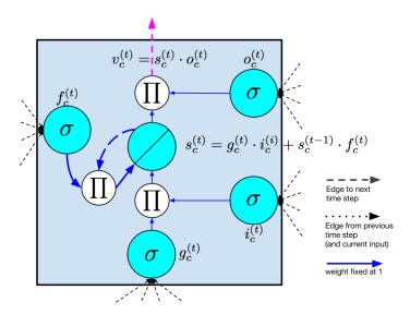
Figure 10: LSTM memory cell with a forget gate as described by Gers et al. [2000].
