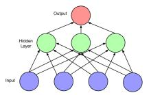
Figure 2: A feedforward neural network. An example is presented to the network by setting the values of the blue (bottom) nodes. The values of the nodes in each layer are computed successively as a function of the prior layers until output is produced at the topmost layer.
