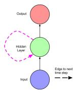
Figure 7: A simple recurrent net with one input unit, one output unit, and one recurrent hidden unit.
