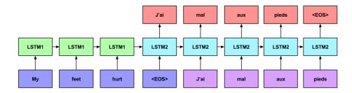
Figure 14: Sequence to sequence LSTM model of Sutskever et al. [2014]. The network consists of an encoding model (first LSTM) and a decoding model (second LSTM). The input blocks (blue and purple) correspond to word vectors, which are fully connected to the corresponding hidden state. Red nodes are softmax outputs. Weights are tied among all encoding steps and among all decoding time steps.
