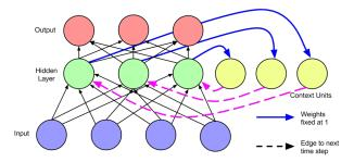
Figure 6: A recurrent neural network as described by Elman [1990]. Hidden units are connected to context units, which feed back into the hidden units at the next time step.
