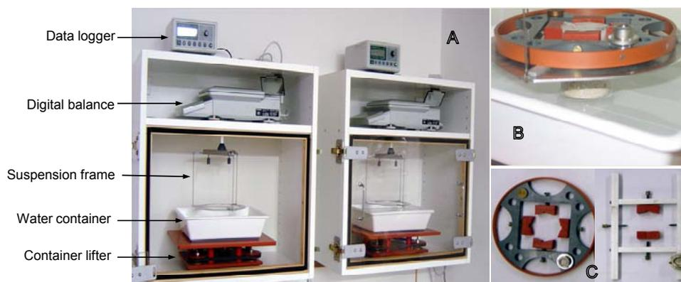
Figure 3-8 Automated water absorption apparatus (A); specimen fixed in specimen holder hanging above the water by suspension frame (B); different types of specimen holders (C)
