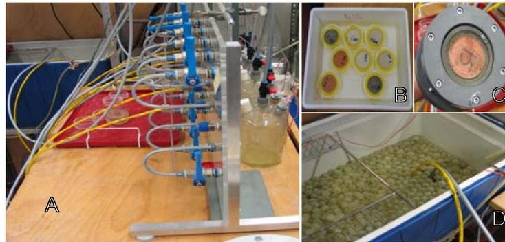
Figure 3-15 Head permeameter apparatus (A); laterally sealed specimens (B); head permeameter with specimen (C); water container (D) (Plagge et al. 2007)
