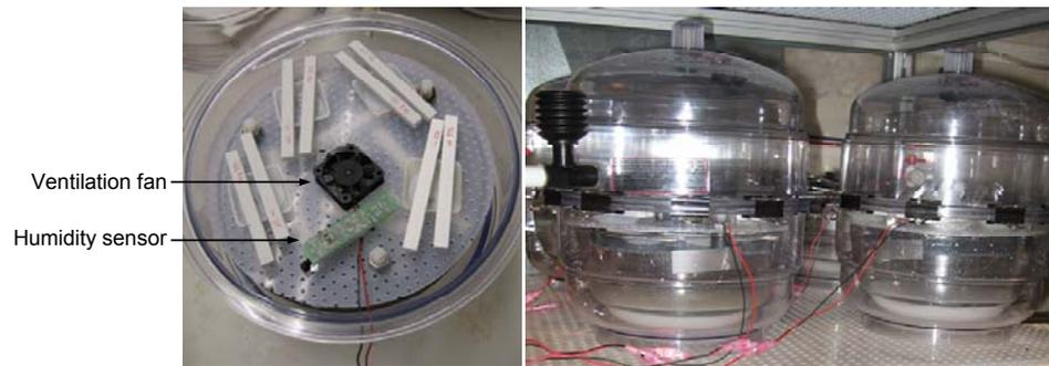
Figure 3-4 Desiccator chambers with the saturated salt-in-water solution
