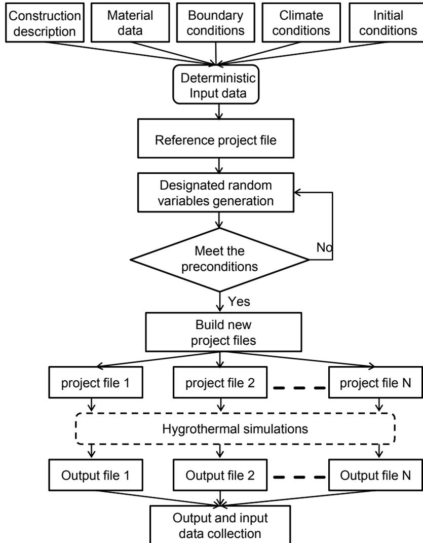
Figure 6-2 Schematic drawing of implementation of uncertainty propagation
