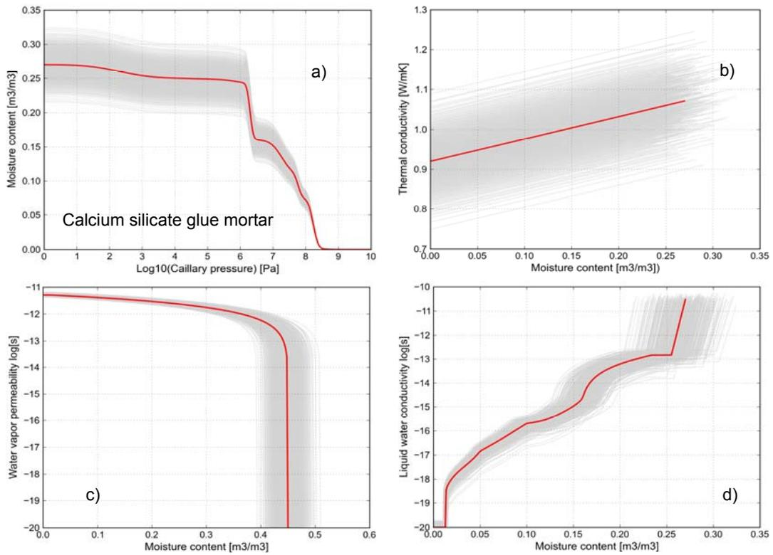
Figure 7-11 Material functions of calcium silicate glue mortar a) moisture retention curve b) thermal conductivity c) water vapor permeability d) liquid water conductivity
