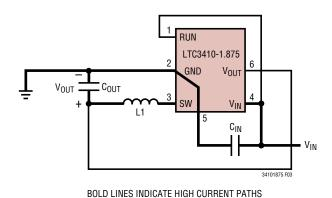
Figure 3. LTC3410-1.875 Layout Diagram
