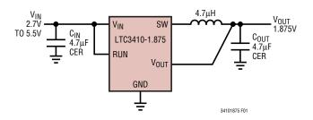
Figure 1. High Efficiency Step-Down Converter
