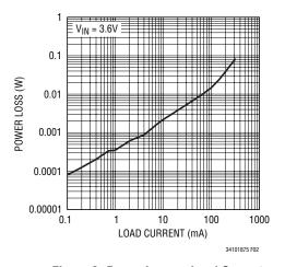
Figure 2. Power Loss vs Load Current
