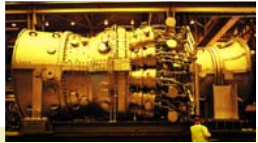
GE Power Systems' new 480-megawatt "H" turbine will be the world's most energy-efficient combined-cycle electricity generator.
