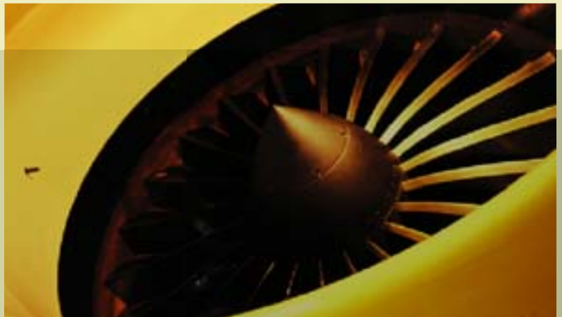
The GE90-115B jet engine, the world's most powerful thrust aircraft engine, has the diameter of a Boeing 737 fuselage.
