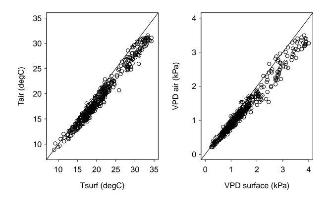
Both surface temperature and VPD are in most cases higher than the ones measured at tower height.
