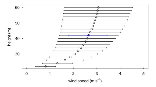
Here, the points denote the mean wind speed and the bars denote the standard deviation. The blue point/bar represent the values that were measured at 42m. In this case we see that the wind speed as "back-calculated" from the wind profile agrees well with the actual measurements.
