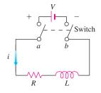
Use a phase line analysis to sketch the solution curve assuming that the switch in the *RL*-circuit is closed at time t = 0. What happens to the current as  $t \rightarrow \infty$ ? This value is called the *steady-state solution*.
