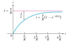
**FIGURE 16.6** The growth of the current in the *RL* circuit in Example 4. *I* is the current's steady-state value. The number t = L/R is the time constant of the circuit. The current gets to within 5% of its steady-state value in 3 time constants (Exercise 31).
