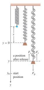
**FIGURE 17.3** The propulsion force (weight)  $F_p$  pulls the mass downward, but the spring restoring force  $F_s$  and frictional force  $F_r$  pull the mass upward. The motion starts at  $y = y_0$  with the mass vibrating up and down.
