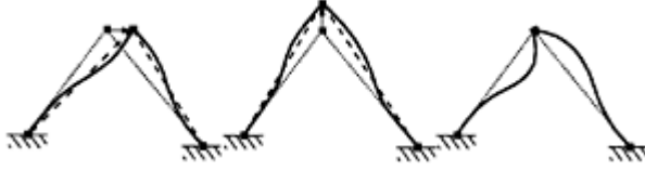
FIGURE 6.6 Compatibility between nodal and element end displacements.
