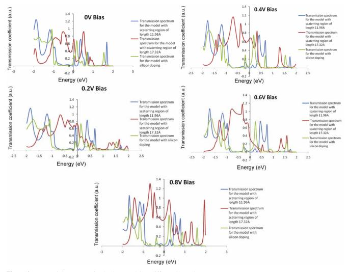
Figure 4. Transmission spectra for the three models at different bias voltages.
