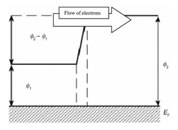
Figure 6. Formation of a metal-metal junction.
