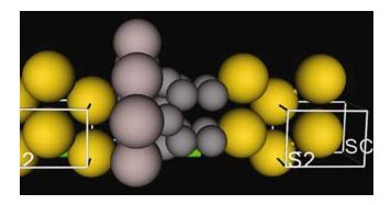
**Figure 1.** Asymmetric metal–CNT structure with central scattering region of length 11.96 Å.
