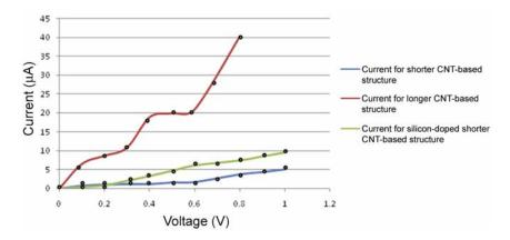
**Figure 5.** I-V characteristics for three asymmetric metal–CNT models. The dots represent the value of current for respective step-bias voltage.
