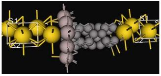
**Figure 3.** Asymmetric metal–CNT structure with central scattering region of length 17.32 Å.
