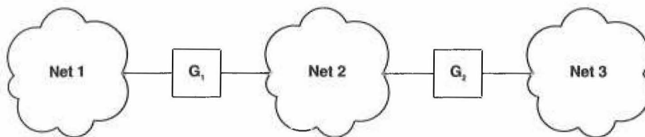
Figure 3.2 Three networks interconnected by two gateways.
