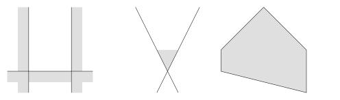
Fig. 1.1: With the objective function being to find the highest point, we have from left-to-right an infeasible linear program, and unbounded linear program and a bounded linear program.
