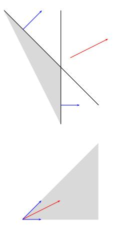
Fig. 3.3: A roof that is defined by the two constraints  $x_1 \le 2$  and  $x_1 + x_2 \le 3$ . The objective function vector is  $(2, 1)^T$ . Indeed  $(1, 1)^T = 1 \cdot (1, 1) + 1 \cdot (1, 0)$  which shows that it is in the cone generated by the constraint-defining vectors.
