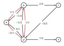
Fig. 6.6: The residual network of the flow in Figure 6.5 and a negative cycle marked by the red edges.
