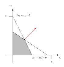
Fig. 1.2: A two-variable linear program
