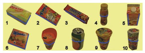
Fig. 11. Ten test objects. The blue lines represent the optimal positions for grasping points near the centre of the objects, depending on the used gripper. From left top: 1. Dextro, 2. Yippy, 3. Snickers, 4. Cafemio, 5. Exotic, 6. Manner, 7. Maroni, 8. Cappy, 9. Smoothie, 10. Koala.
