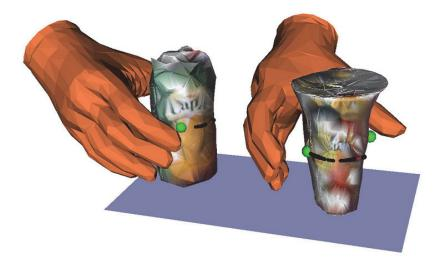
Fig. 9. The rotation axis of the hand is defined by the fingertip of the thumb and the index finger of the gripper. This rotation axis must be aligned with the axis defined by the grasping points. The calculated grasping pose of the gripper is by object no. 8 (Cappy) -32.5° and object no. 9 (Smoothie) -55°.
